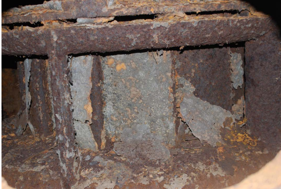
Figure 6. Headcover, Stay Vanes and Wicket Gate Assembly
